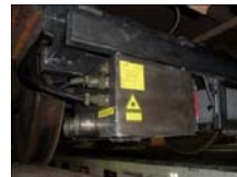
6. Laser profiler and inertial pack for track geometry monitoring
