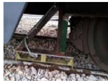
5. Eddy Current distance sensor & accelerometers
