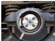
4. Hollow shaft acoustic system
