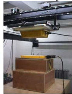
SIEMENS EUROBALISE test bench In Braunschweig
