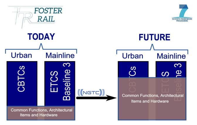
Based on the NGTC FRS the project is now developing the system architectures, functional allocation, and interfaces (FIS) for a next generation of train control systems for the mainline and urban markets. These new architectures will utilise a common ATO, while maintaining the separate urban and mainline ATPs. Work on the common ATO are using as an input the results from the: MODURBAN project (a previous FP6 project); and the ATO over ETCS project (part of TEN-T program).
